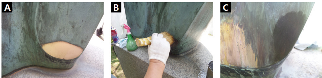
Figure 6. Patination test. (A) After polishing the surface, (B) The patination process, (C) After the coating process.
